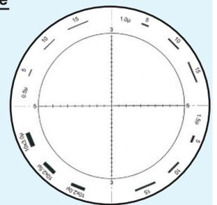
**IMPORTANT NOTE.** The circle on these Walton & Beckett reticles must represent 100 microns at the stage and each one must be manufactured to suit the individual instrument. Therefore, details should be provided with your order of :- Calibration factor, if known or Objective magnification, eyepiece magnification, diameter of reticle disc required, microscope make and model.
