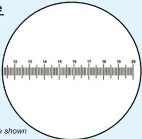
NE1 Scale: This eyepiece reticle has an overall length of 10.00mm with 100 subdivisions of 0.1mm. When used with a x10 objective each division will represent 10 microns on the specimen. By dividing the division of the chosen reticle by the magnification of the objective one obtains an approximate value that each division will represent on the stage.
